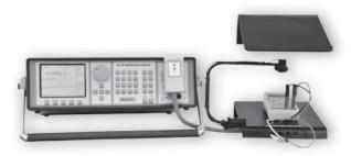
CamOcr camera module extends possibilities of MEATEST automatic calibration software Caliber by scanning readouts directly from 7 segment digital displays. CamOCR can do any number of repeated measurements, decreasing type "A" uncertainty.
