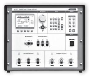
Outstanding accuracy and resolution are quite common for Meatest instruments but the best thing about M133C is its flexibility. All three phases are completely independent and AC signal can be set up in many different ways including phase shift, frequency, harmonic and interharmonic distortion, amplitude modulation by yet another independent signal and dip/swell.
