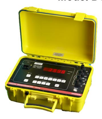
The DO7e is a very rugged yet compact and portable digital microhmmeter for the measurement of low resistance. Using a rechargeable sealed lead acid battery with built-in charger, the DO7e is capable of measuring with a current of 10Amps on the lowest range.
