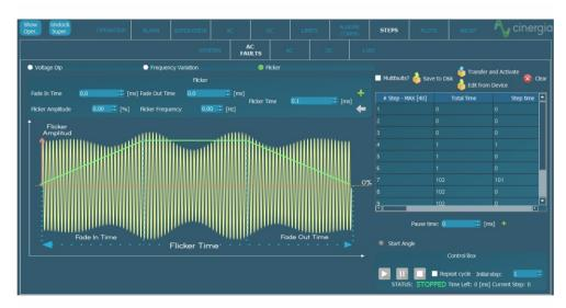
Disturbance Generation The steps mode includes predefined easy-to-use test panels. The AC faults panel is a powerful yet intuitive editor which allows generating and configuring voltage dips, frequency variation, flicker and LVRT. Specific profiles can be saved in .csv files, modified, and reused by importing an existing one. The LVRT page have predetermined profiles for differents countries.
