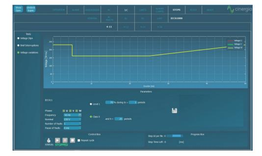
IEC Testing (option) The last version of software includes a library supporting IEC compatible tests. The profiles defined in the standards are preloaded in the software for a user friendly execution and edition. Currently the following standards are available:
